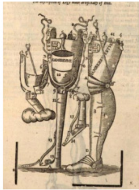
Figure 25: A more complex artificial leg “of iron,” with its multiple layers shown, from 587 of The Workes of that Famous Chirurgion , Ambroise Parè. Source: Wellcome Collection.
