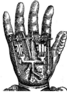
Figure 27: A surprisingly complex mechanism for a prosthetic hand, called Le Petit Lorrain , from 916 of Les Oeuvres d'Ambroise Paré , 1633 edition.
